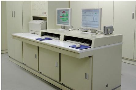
Diagnostic Tools for ATP/TD and Interlocking Equipment are aimed to support maintenance work by constantly monitoring the states of power supplies and railway signaling systems such as ATP/TD wayside equipment, and electronic interlocking. Also, in case of trouble, the abnormal locations are displayed in the image of racks and equipment. In addition, the operating state of each equipment is stored at all times for defect analysis after restoration.
