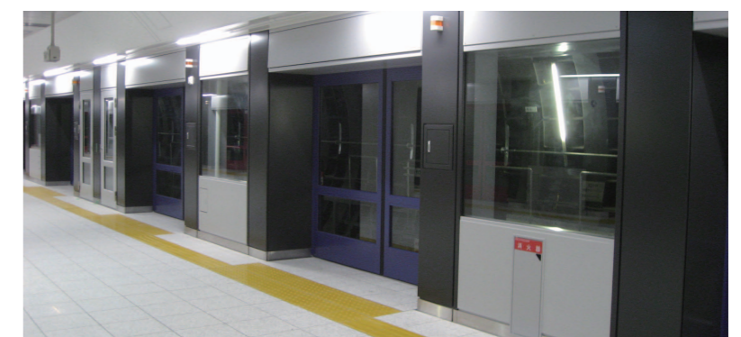
Installation Example of the Full-screen Doors
